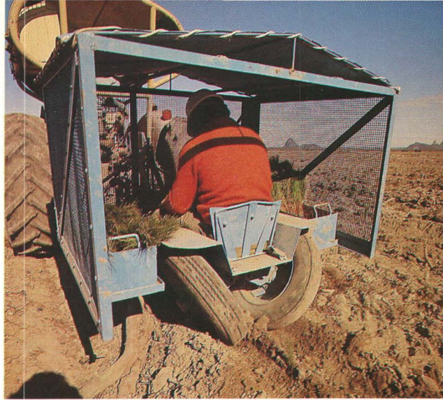
Oddly-angled wheels ensure good soil compaction around newly-planted pine seedlings, Beerburrum
